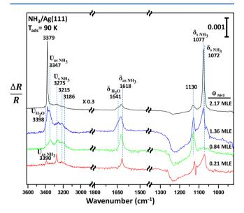
**Figure 5.** IRAS spectra of ammonia adsorption on a clean Ag(111) surface at 90 K as a function of the ammonia surface coverage.
