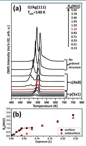
**Figure 1.** (a) TPD profiles for oxygen desorption (m/z = 32) obtained by increasing ozone exposures on clean Ag(111) at 140 K. (b) Relative oxygen surface coverages (obtained via integrated TPD desorption signals in part a) for surface and subsurface oxygen species on Ag(111) as a function of the ozone exposure.
