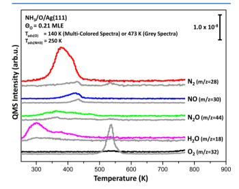
Figure 6. TPRS profiles for the reaction of ammonia with oxygen on Ag(111). In all of the experiments, an identical exposure of NH<sub>3</sub> ( $P_{NH_3}$ =  $2.0 \times 10^{-9}$  Torr  $\times 60$  s) was dosed at 250 K on an oxygen-covered  $(\theta_{\rm O} = 0.21 \text{ MLE}) \text{ Ag}(111)$  surface, where oxygen was delivered by ozone exposure either at 140 K (multicolored spectra) or at 473 K (gray-colored spectra).
