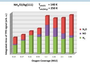
**Figure 8.** Integrated TPD desorption signals for the main ammonia SCO products (i.e.,  $N_2$ , NO, and  $N_2$ O) on an O/Ag(111) surface as a function of the oxygen coverage extracted from the TPRS data given in Figure 7. See the text for details.
