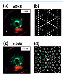
**Figure 2.** LEED images of O/Ag(111) overlayers obtained by introducing different ozone exposures at 140 K on a clean Ag(111) surface followed by pumping and annealing to 473 K in UHV. (a) LEED image of the p(5×1)-O/Ag(111) overlayer ( $\theta_{\rm O}$  = 0.83 MLE) and (b) its simulated (theoretical) LEED pattern. (c) LEED image of the c(4×8)-O/Ag(111) overlayer ( $\theta_{\rm O}$  = 1.10 MLE) and (d) its simulated (theoretical) LEED pattern.
