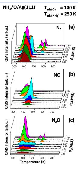
**Figure 7.** TPRS profiles of various ammonia SCO reaction products (i.e.,  $N_2$ , NO, and  $N_2$ O) for the reaction between ammonia and oxygen-precovered Ag(111) surfaces as a function of the oxygen coverage. For all of the data, oxygen was delivered on Ag(111) by ozone exposure at 140 K, while NH<sub>3</sub> was delivered using an identical ammonia exposure at 250 K ( $P_{\rm NH_3} = 2.0 \times 10^{-9} \, {\rm Torr} \times 60 \, {\rm s}$ ).
